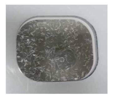
With the hole successfully cut and removed, leave the template in place as this will be the guide for the roundover bit.
