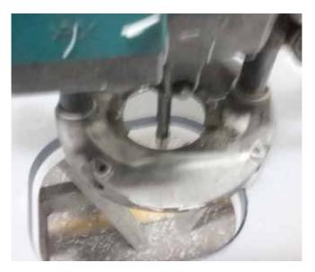
Always run the router clockwise when using the template to cut. Flush rout the camera hole to the camera hole template.
