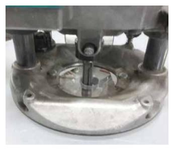
Bearings must line up with template on the bottom of the acrylic.
