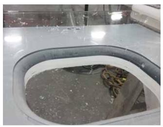
Router to the camera hole template using the roundover bit. The bearing should run entirely on the camera hole template.
