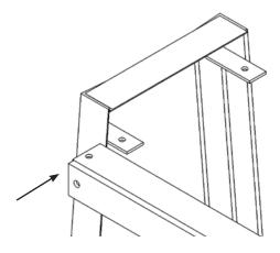
4. Tighten all 3/8" fasteners put in place during steps 3 and 4 using a 9/16" wrench and socket.
