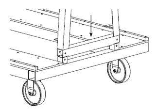
3. Place cross members between A-Frame ends as shown. Fasten in place to flatbar gussets using 3/8" x 1" hex bolts, 3/8" flat washers and 3/8" Nylon lock nuts provided. Repeat for all 6 cross member pieces.
